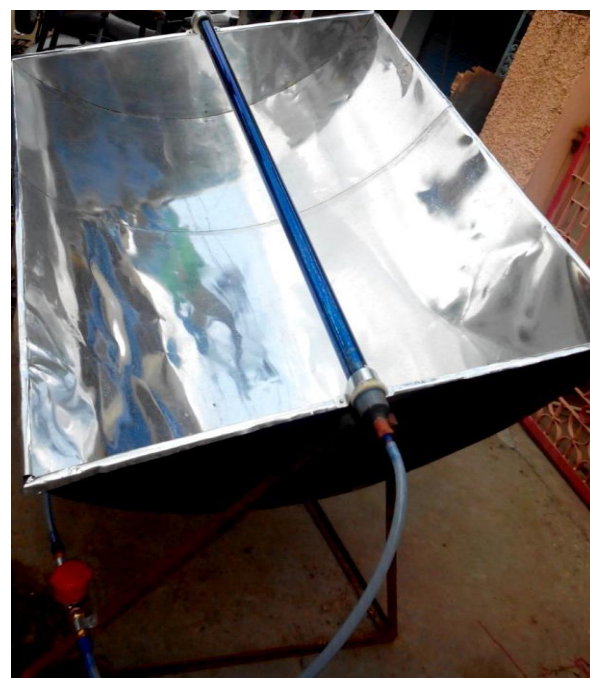
Fig 2: Fabricated model of solar parabolic trough system
